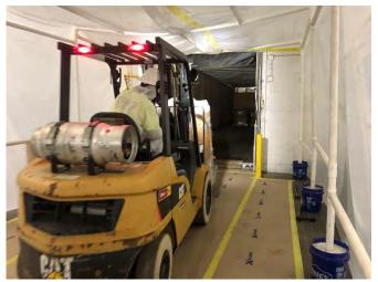
Processed material is loaded single-stack onto a parked trailer through the contaminant reduction zone for Novotec Recycling.
