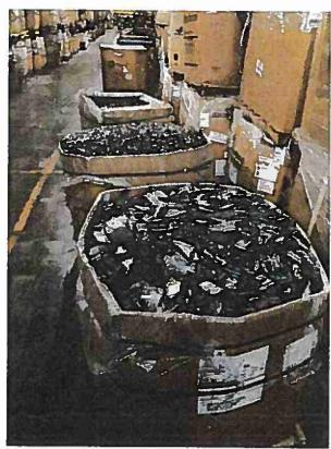
View of a typical container of crushed CRT glass.
