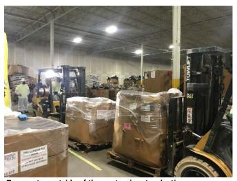
Tow-motor outside of the contaminant reduction zone passes processed material to the clean loading tow-motor within the CRZ.
