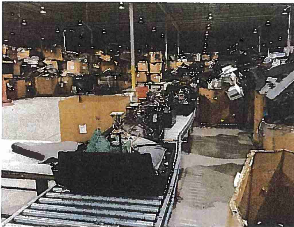
View of a manual processing line in the south portion of building 1675 where TVs and computer monitors would be disassembled.
