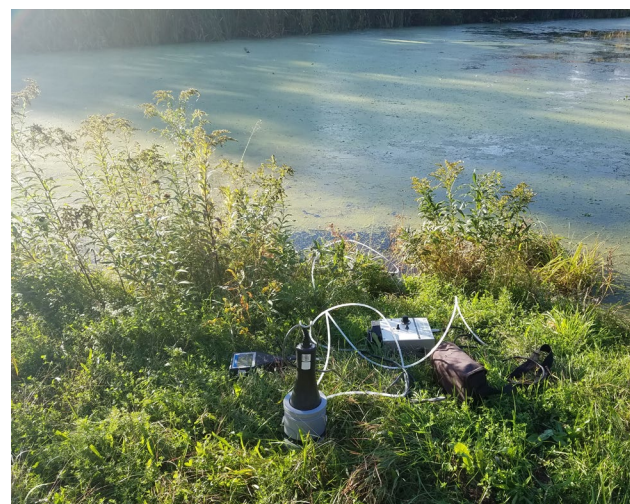
Field sampling requires PFAS-specific SOPs to ensure data quality and minimize the chances of cross contamination from ubiquitous PFAS sources.
